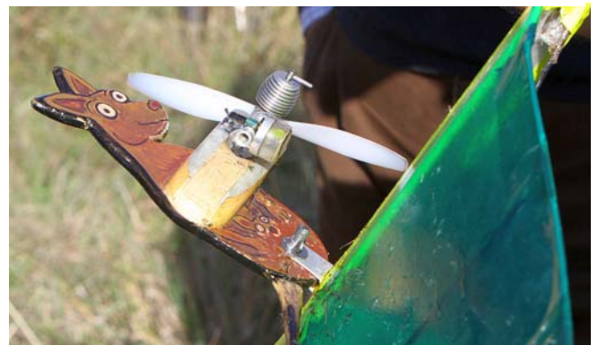
Fig. 6 Stowe's Kanga, showing (above), its robust wing structure and (above right) unique "Australian" profile: 'roos and beer. Note the thin, reflexed airfoil of this flying wing model, quite stable in spite of lack of dihedral. (right) Mills 0.75 is side-mounted on the kangaroo pylon, adjustable for downthrust.
