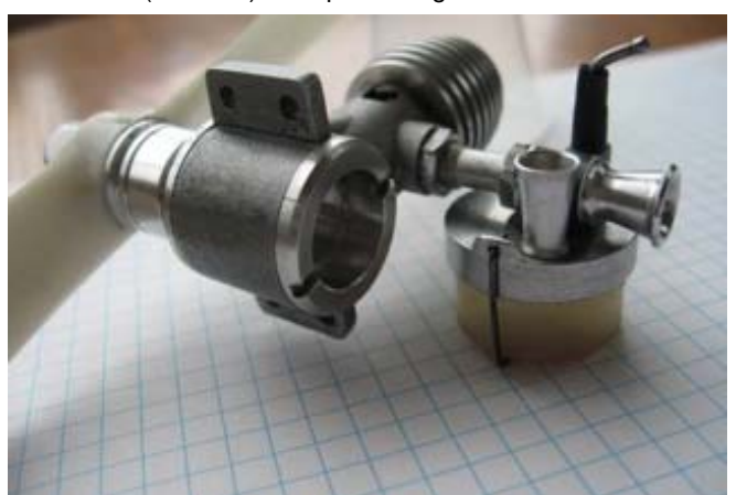
Fig. 7 (above) Modified Mills 0.75 cc used by author, note special BB front end. (below) New induction and tank system, with peripheral jet carburetor (a la Cox) and quick filling device.
